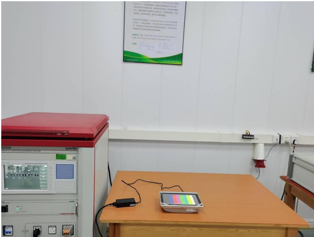
Test Setup Photo of Harmonic & Flicker Measurement
