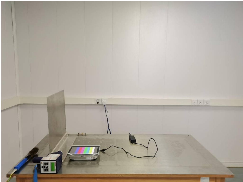
Test Setup Photo of Electrostatic Discharge Test
