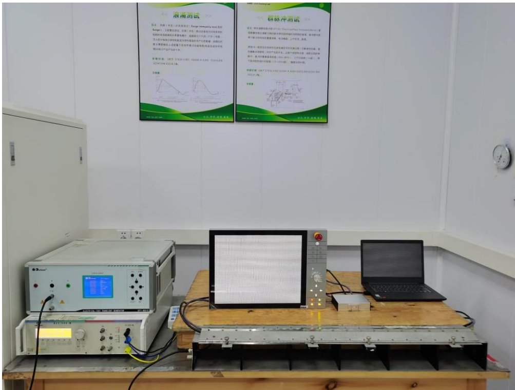
Photo of Singal port Electrical Fast Transient/Burst Test Immunity Test
