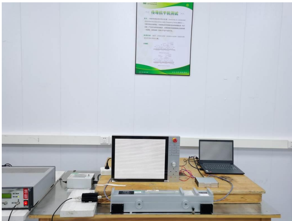
Test Setup Photo of Singal Port Injected Currents Susceptibility Test
