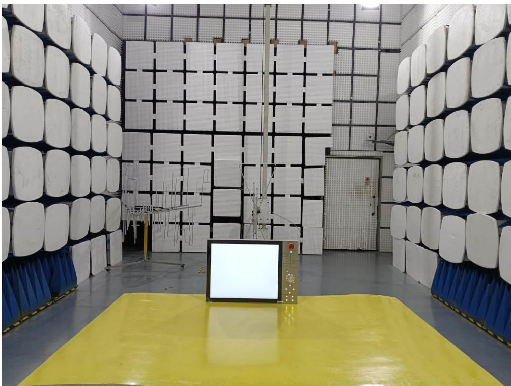
Test Setup Photo of Radiated Measurement (30MHz~1GHz)
