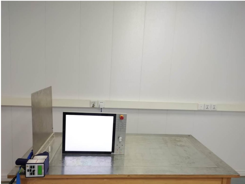
Test Setup Photo of Electrostatic Discharge Test
