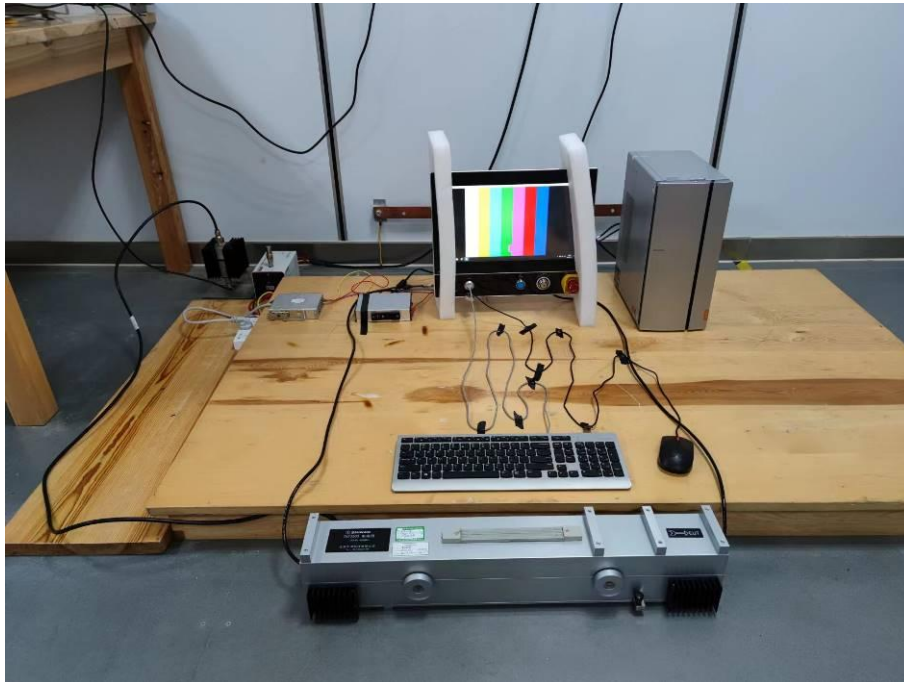
IEC 61000-4-6 CS Immunity Test View(signal port)
