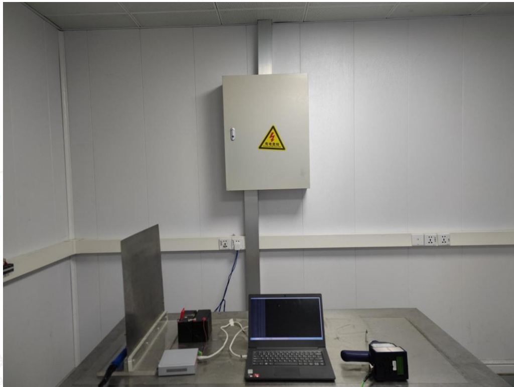
Test Setup Photo of Electrostatic Discharge Test
