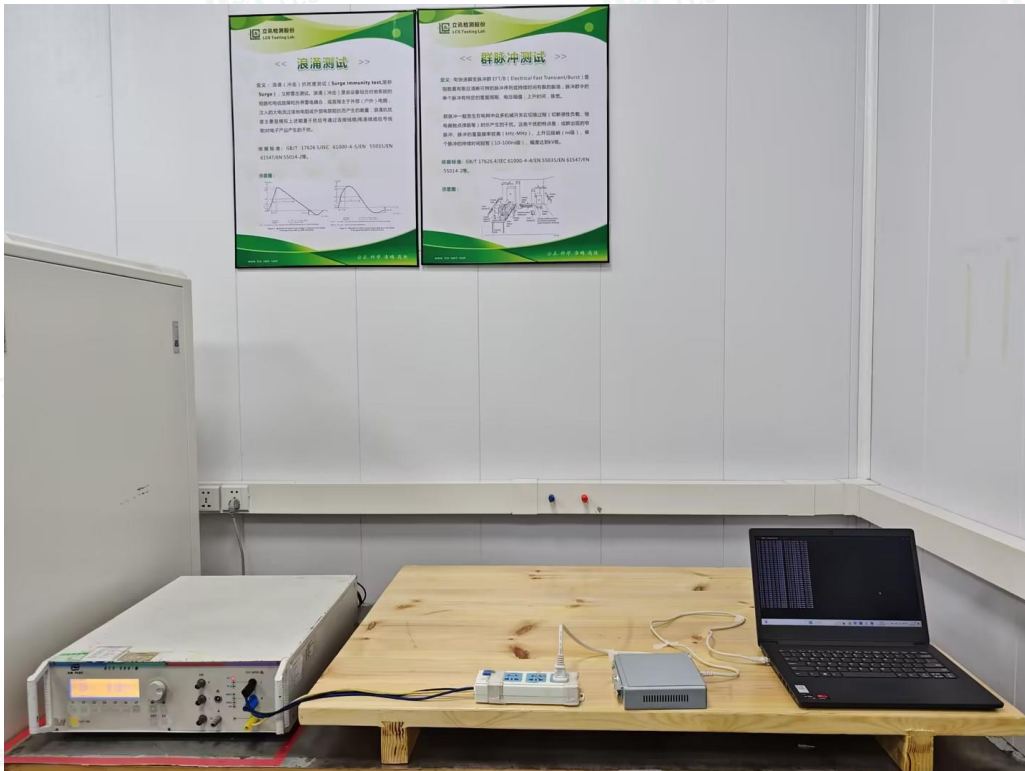
Photo of Electrical Fast Transient/Burst Test &amp; Surge Immunity Test
