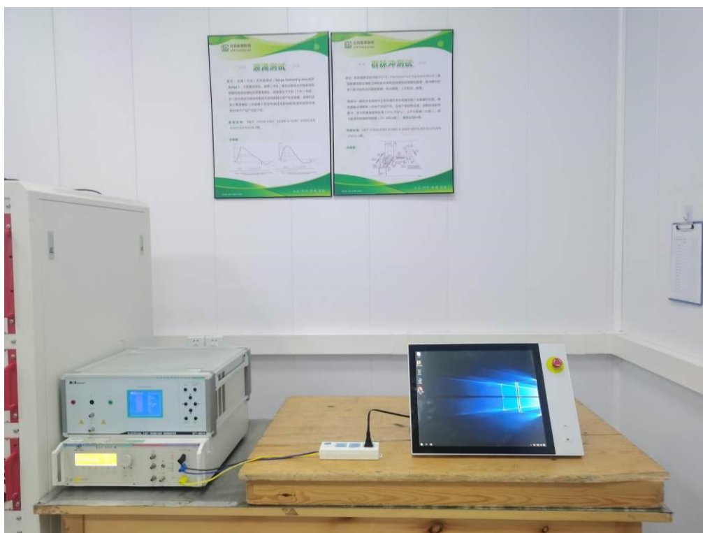
Photo of Power Line Electrical Fast Transient/Burst Test & Surge Immunity Test
