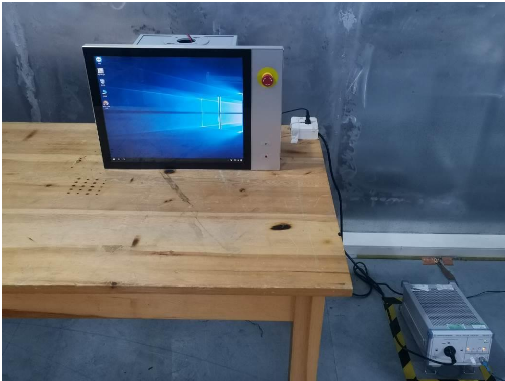
Test Setup Photo of Power Line Conducted Measurement
